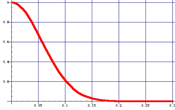
Figure 4.1: The damping factor e^{-\frac{\sigma^2 \Delta m^2}{2}} as function of the proper time error \sigma . The time resolution can reduce significantly the A_{CP} amplitude. The present mean value for the proper time error in LHCb is estimated about \sim 40 fs and for this reason the damping factor is still quite close to 0.8. Otherwise an error value near \sim 100 fs will reduce outrageously the A_{CP} amplitude.
