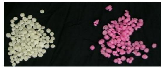
Fig. 10. Bioplastic granules before (left) and after imbibition with MDRB
