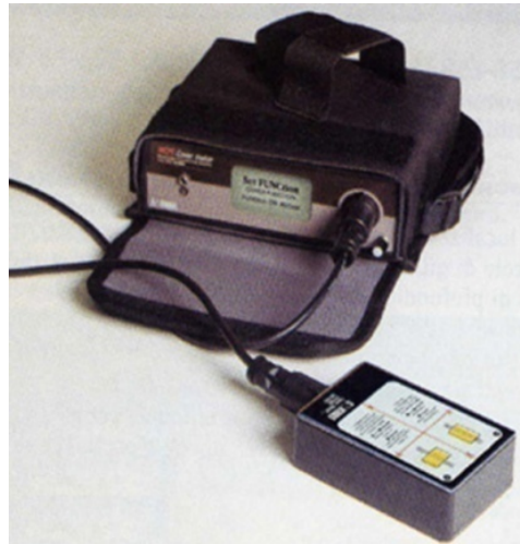
Fig. 2.3. A covermeter survey equipment used to locate reinforcement.
