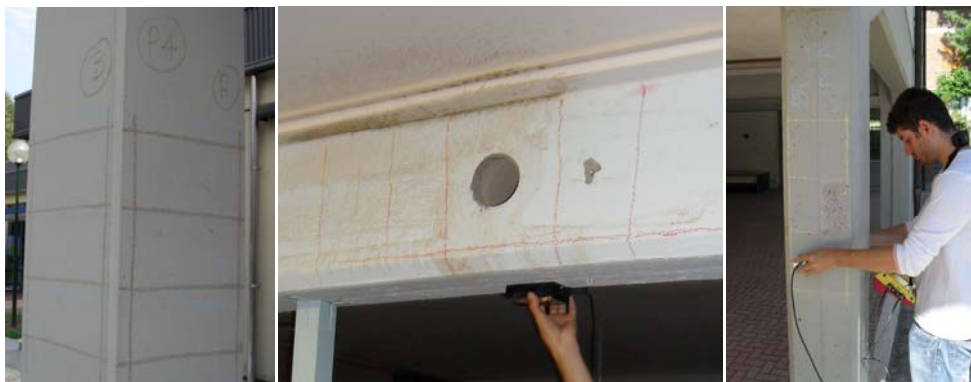
Fig. 2.2. Different aims for a covermeter survey: a) to estimate the actual arrangement, number and diameter of reinforcing bars; b) to identify concrete areas on which drilling core samples; c) to identify concrete areas on which carrying out NDT methods.
