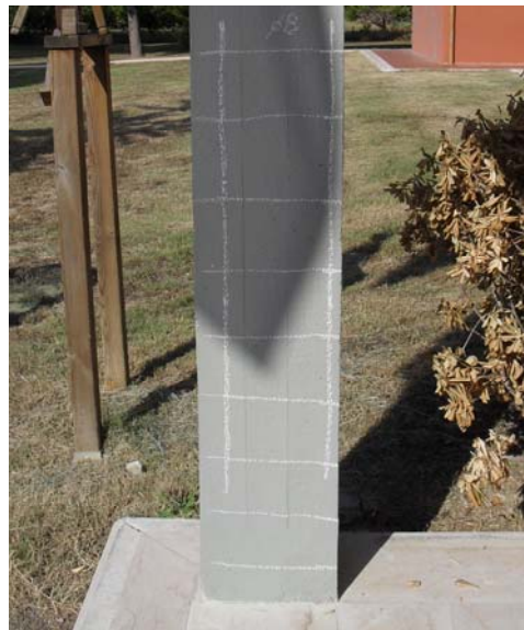
Fig. 2.4. A covermeter survey on the surface to be investigated.
