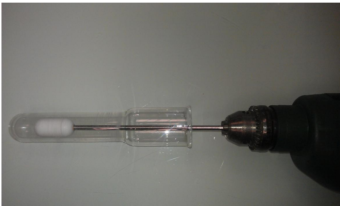
Fig. 6 Potter-Elvehjem tissue grinder tube with PTFE piston used for shellfish tissue grinding.
