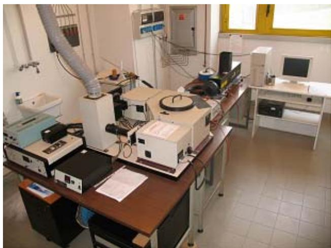
*Edinburgh FLS920 spectrometer equipped with an integrating sphere-laser setup*
