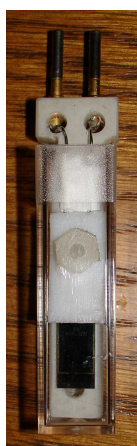
Figure 18. This cell allows connection of chip miniaturized contacts with electrochemical instrument without soldering.
