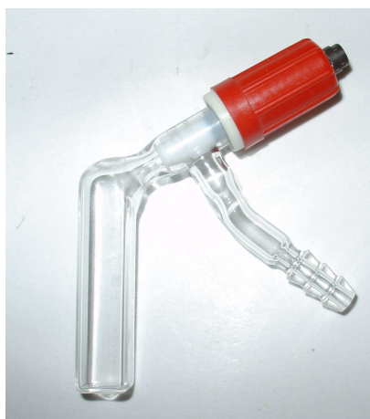
Figure 11. Homemade cuvette intended for fluorescence experiments in vacuum or degassed solutions.
