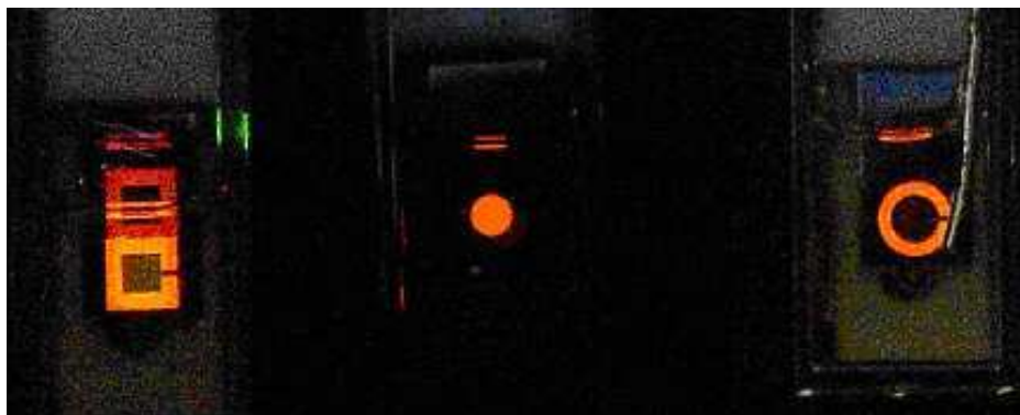
Figure 13. Photographic images of ECL emission from a 0.1 mM Ru(bpy) 3 2+ / 3x10 -2 M NPr 3 solution. Supporting electrolyte: 0.1 M PBS at pH 7.5. From the left to right: EQ_2000_5, EC_2000_5 and again EC_2000_5 chip electrode. ECL emission appears homogeneous in all working electrode surface. These images show the possibility to invert the counter with working electrode by retaining the emission.
