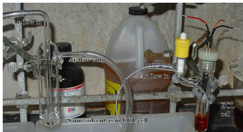
Figure 7. The ECL cell geometry allows an accurate degassing of solution by a 5 minutes Ar bubbling and exposure of the sample to air when required. Ar is saturated with solvent vapours to avoid his evaporation from sample.
