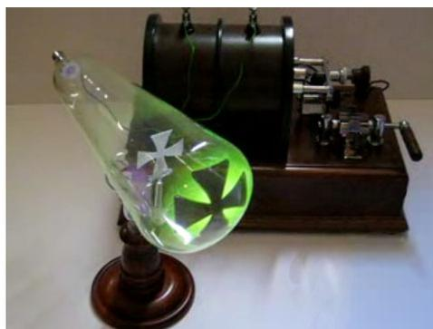
**Figure 1.1:** Crookes tube and power generation system.
