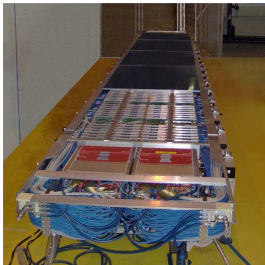
Figure 2.24: A TOF SM after the assembly of the 5 modules. Two of the four crates are visible (the other two are on the opposite side). These crates house the readout and control electronics. The top aluminium covers enclose completely the front-end electronics placed on the modules.
