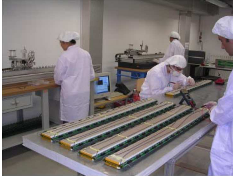
Figure 2.19: MRPCs production at Bologna-INFN laboratories.
