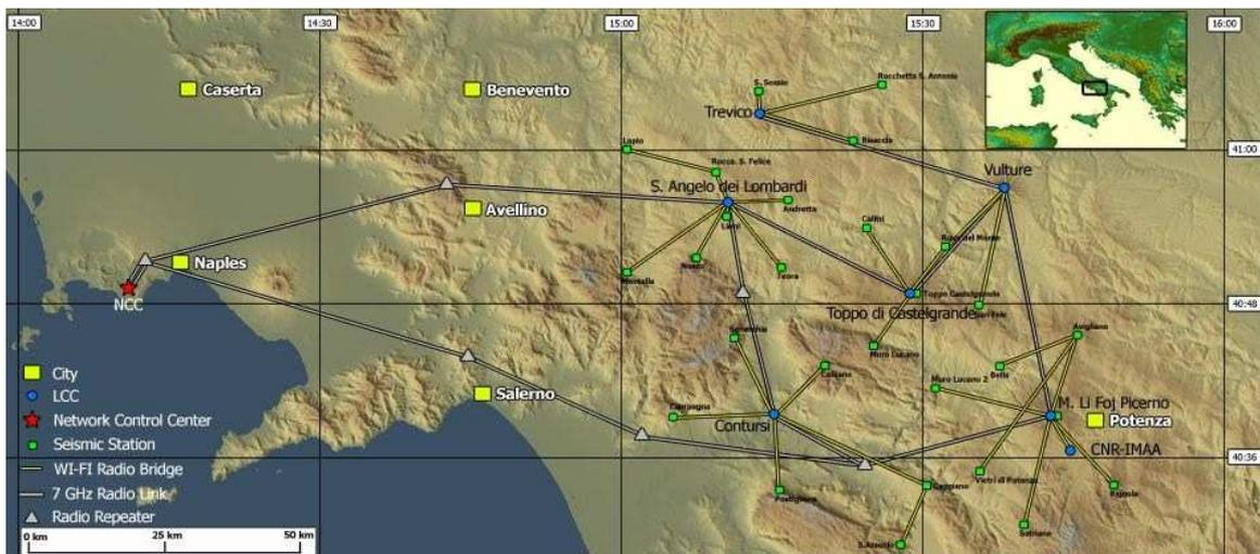
Figure 1.3: Green squares indicate seismic stations. Yellow lines symbolize wireless radio links between each seismic station and its nearest Local Control Center (LCC, blue circles). Gray lines represent higher bandwidth, wireless connections among LCCs and the Network Control Center (red star). The latter transmission system is conceived as a redundant double ring.
