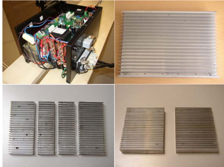
Fig. 2. Clockwise from top left: SMPS voltage regulator used in the tests; original single heatsink; two heatsinks; four heatsinks.
