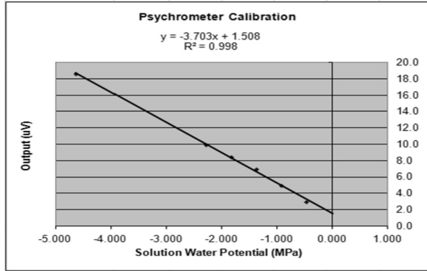
Fig. 4-3 Linear relationship between uV output and NaCl concentration in the calibration solution
