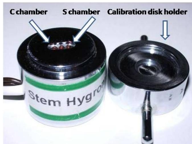
**Fig. 4-4 Stem Psychrometer picture with indication of the position of the two chamber and of the calibration disk holder.**
