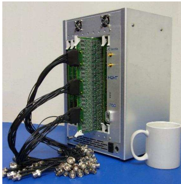
Fig. 65 – Tecella Apollo 384ch Patch Clamp Amplifier (from Tecella product catalogue).
