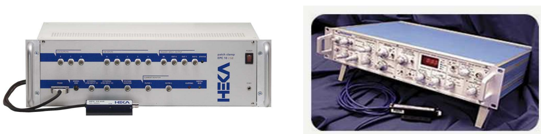
Fig. 14 – On market available patch clamp amplifier: HEKA EPC 10, Axon Axopatch 200b.
