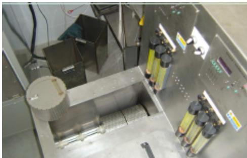
*Fig. 4.2.1 - Independent steeping/germination tanks with the four drums*
