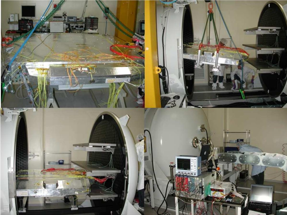
**Figure 3.13:** Pictures of the LTOF during TVT test in Terni documenting its insertion in the SERMS TVT chamber.
