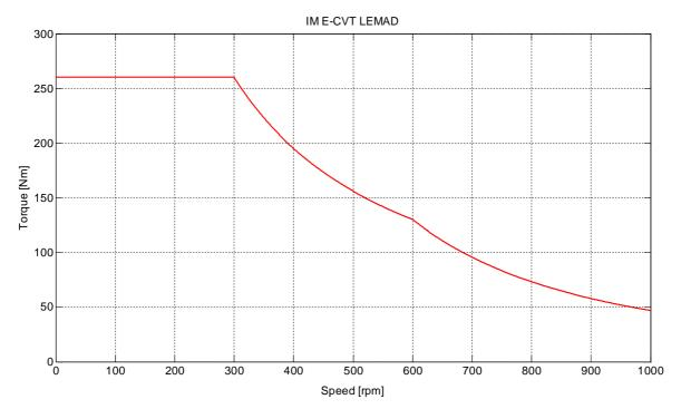
Fig. 5.7 – Induction machine torque limit characteristic
