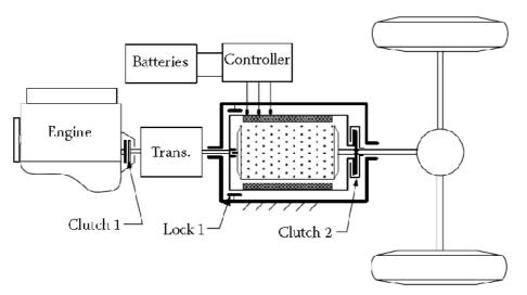
*Fig. 1.12 –Parallel hybrid driveline - speed coupling with transmotor*
