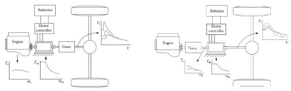
Fig. 1.9 –Parallel hybrid drivetrain- torque coupling – single shaft a. Before transmission b. After transmission
