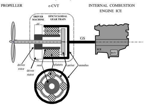
Fig. 3.1- Scheme of the power split e-CVT for hybrid ship propulsion
