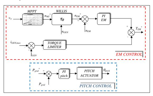
Fig. 4.11 – WT-CVT control system layout
