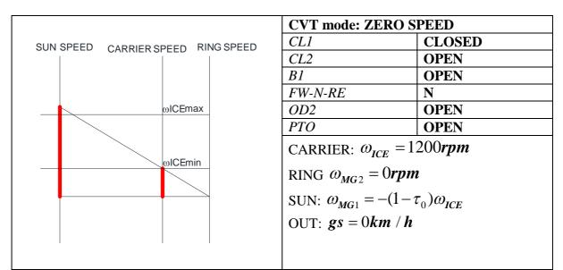
*Fig. 2.6 - Zero speed ICE start-up: monogram, speed relationships and mechanical configuration*
