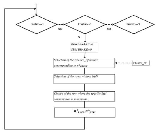
Fig. 3.19- Flow chart for operating mode 3: MIN\_CONS\_1
