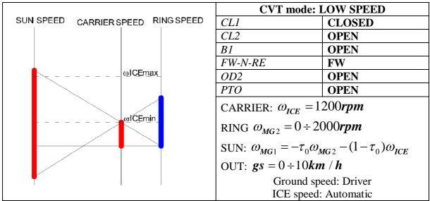
*Fig.* 2.5 – *CVT mode, low output speed, cinematic nomogram, speed relationships and mechanical configuration*
