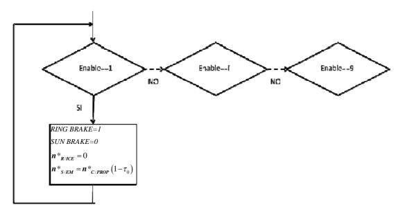
Fig. 3.18- Flow chart for operating mode 1: ONLY\_EM
