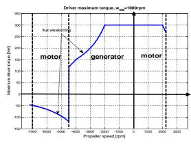
Fig. 3.12 Output torque of the driver EM vs. driver speed for  $\boldsymbol{\omega}_{\mathbf{R},\mathbf{ICE}} = 1000 \ [rpm]$
