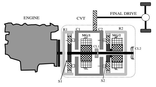
Fig. 1.15 – Scheme of compound power split e-CVT
