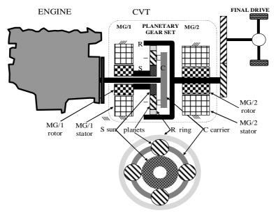
Fig. 1.13 – Scheme of the input power split e-CVT
