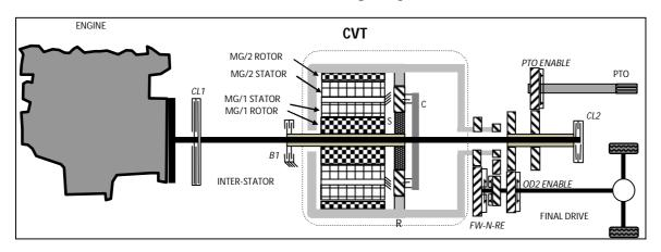
• *B1* allows to block the sun shaft, imposing a fixed ratio between ICE and CVT
