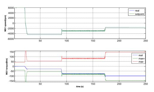
*Fig.* 2.30 – *Simulation 3, MG/1 speed and torque*
