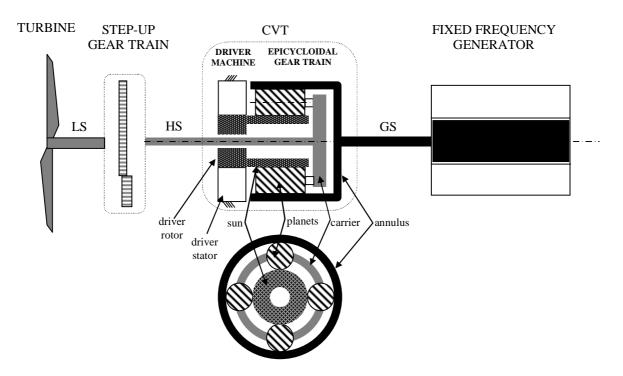
Fig. 4.4- Mechanical layout of the power split e-CVT for Wind Turbine
