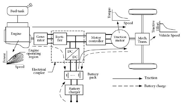
Fig. 1.7 – Series hybrid drivetrain
