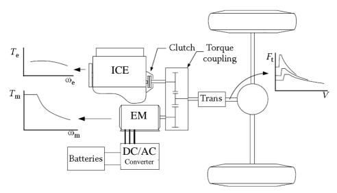
Fig. 1.8 – Parallel hybrid drivetrain (two shafts)
