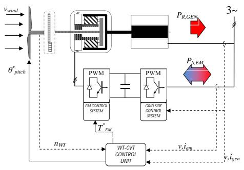
Fig. 4.5- Electrical layout of the power split e-CVT for Wind Turbine (back to back converter)
