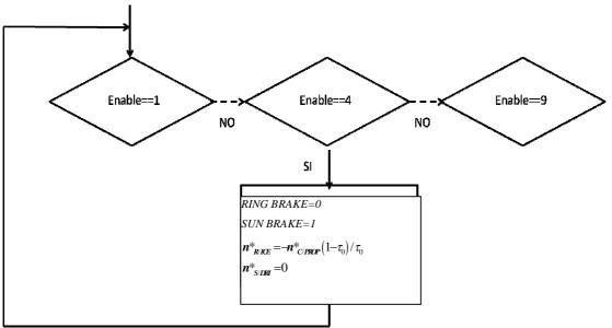
Fig. 3.20- Flow chart for operating mode 4: ONLY\_ICE\_1
