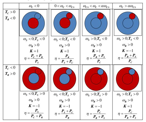
Tab. 1.1 – Operating conditions and efficiencies of the planetary gear set for  $\omega_R > 0$
