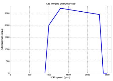
Fig. 3.8- MAN R6-800 full load torque curve
