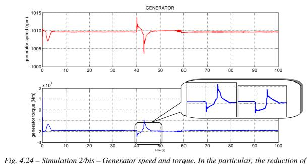
Fig. 4.24 – Simulation 2/bis – Generator speed and torque. In the particular, the reduction of the overload torque compared to the unlimited case.
