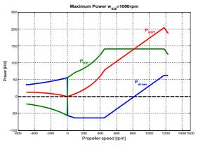
Fig. 3.13 - Maximum power in the three element of the transmission vs. propeller speed for  $\omega$ ICE=1000 [rpm]. P<sub>ICE</sub>: output power of the ICE; P<sub>driver</sub>: output power of the driver; P<sub>OUT</sub>: output power at the propeller shaft.
