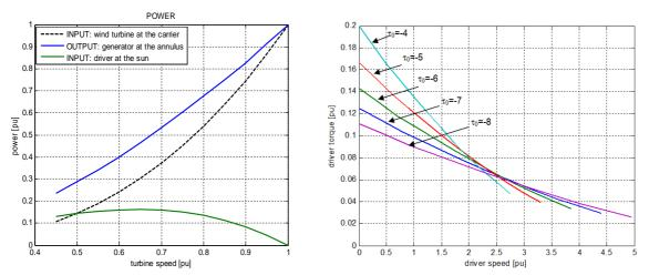
Fig. 4.7 – a) p.u. power curves at MPPT - b) driver torque characteristics at a variable  $\tau_0$ for  $\hat{\omega}_{c_0} = 1$  and  $\hat{\omega}_{R} = 1,143$
