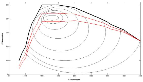
Fig. 2.8- ICE torque characteristic and efficiency map
