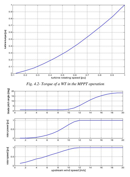
Fig. 4.3- a. Pitch angle, b. Rotor power, c. Rotor speed at a variable wind speed
