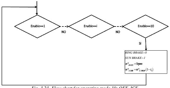
Fig. 3.23- Flow chart for operating mode 10: OFF\_ICE
