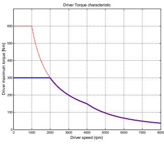
Fig. 3.9- Driver machine torque limit curve
