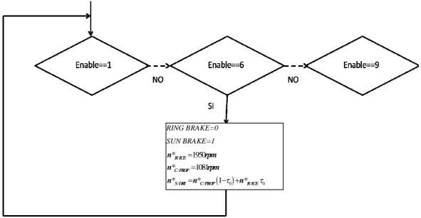
Fig. 3.22- Flow chart for operating mode 6: RECHARGING\_MODE\_2
