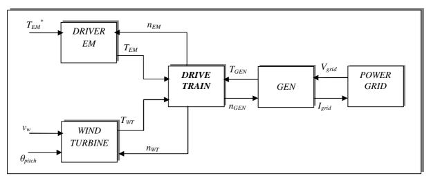
Fig. 4.9 – Block scheme of the WT-CVT system model
