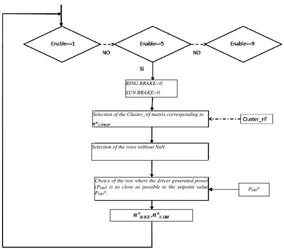
Fig. 3.21- Flow chart for operating mode 5: RECHARGING\_MODE\_1
