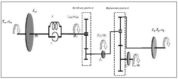
Fig. 1.4 – Scheme of the complete E-CVT transmission model
