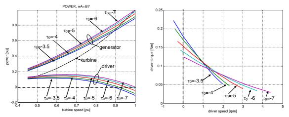
Fig. 4.8 – a) p.u. power curves at MPPT - b) driver torque characteristics at a variable  $\tau_0$ for  $\hat{\omega}_{c0} < 1$  and  $\hat{\omega}_{R} = 1,143$
