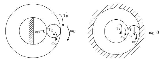
*Fig.* 1.3 – *Torques and speeds of the planetary gear. a) SUN blocked. b) RING blocked.*
