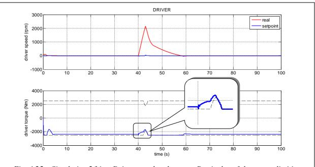
*Fig.* 4.25 – *Simulation 2/bis – Driver speed and torque. Particular of the torque limiting action*
