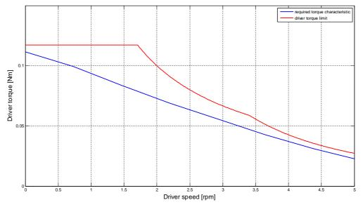
*Fig.* 4.10 – *Driver torque characteristic* ( $\tau_0$ =-8)
