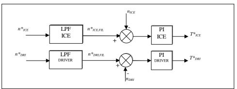
Fig. 3.24- Speed control loop
