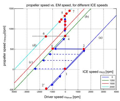
Fig. 3.4- Relationships between speeds in E-CVT power split
