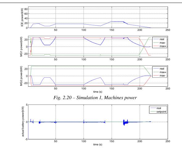
Fig. 2.21 – Simulation 1, Battery power
