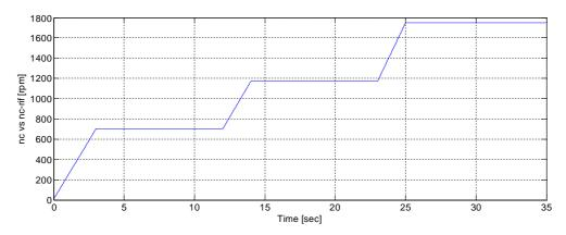
Fig. 3.62- Propeller speed profile
