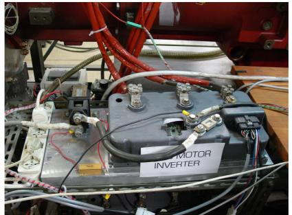
Fig. 5.3 – Particular of the VSI inverter
