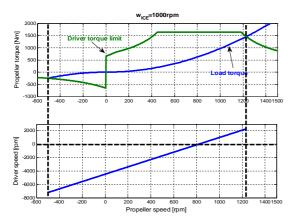
Fig. 3.10. Upper: Output torque of the transmission and load propeller torque vs. propeller shaft speed. Bottom: speed of the driver vs. propeller shaft speed. *Φ*<sub>R,ICE</sub>=1000 [rpm].
