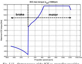
Fig. 3.11 - Output torque of the ICE vs. propeller speed for  $\omega_{R,ICE}=1000 \ [rpm]$
