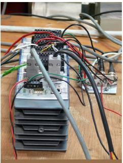
Fig. 5.5 – The CRIO used in lab
