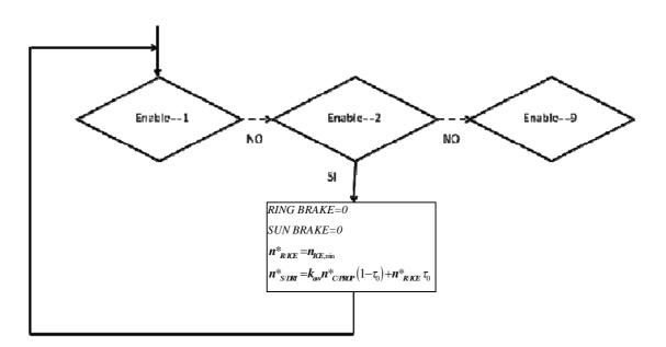
Fig. 3.17- Flow chart for operating mode 2: START\_ICE
