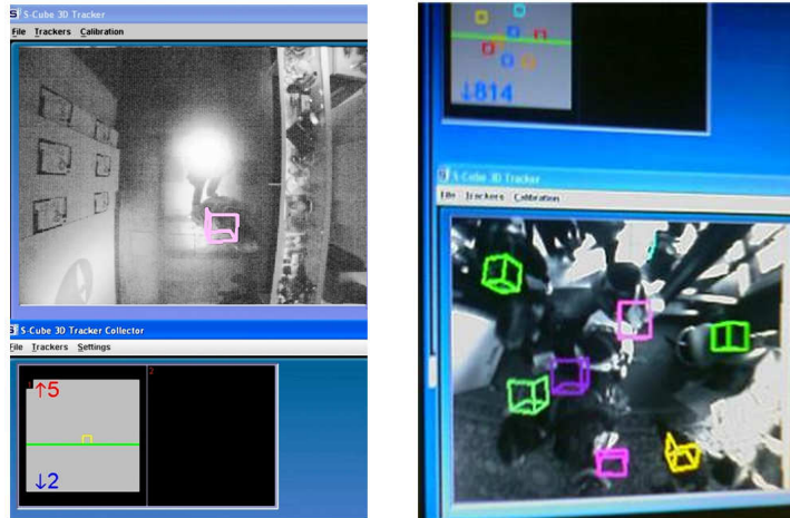
Figure 17: VTS program screenshots. People under the stereo camera are tagged with a colored cube. The VTS counts the people crossing the green virtual line
