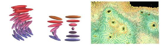
Figure 12: Schematic view of the helical director configuration and mesophase microphotograph between crossed polarized.
