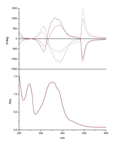
Figure 16: UV-Vis spectra (bottom) and CD (up) of irradiated films of Poly[M6A]-24 (—), and Star[M6A]-24 (—) irradiated with r-CPL (straight line) or l-CPL (dashed line).
