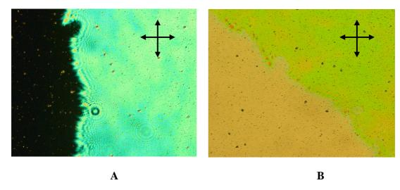
Figure 17: POM textures of a planar-cell filled with Poly[M6A]-24. The right part has been irradiated with r-CPL for 30 minutes. (A) Crossed polarizers parallel and perpendicular to the alignment director: the irradiated zone exhibits a colour while the non irradiated zone is dark. (B) Crossed polarizers rotated of  $45^{\circ}$  with respect to the mesogen director: two different colours are still visible.
