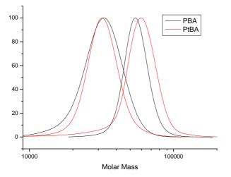
Figure 21: GPC chromatograms of the deprotected PBA and PtBA synthesized
