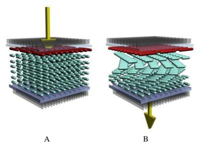
Figure 15: idealization of a LC cell driven by a photochromic command surface. A) linear alignment B) twisted nematic alignment.
