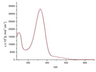
Figure 18: UV-Vis spectra of (S)-ML6A-C (-) and Poly[(S)-ML6A-C] (-).
