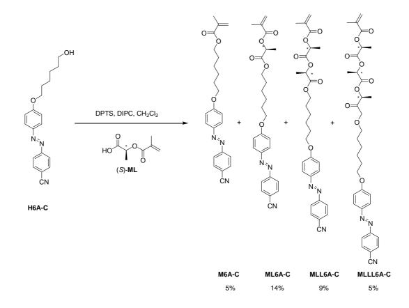
The new monomer (S)-ML6A-C has been synthesized as (S)-ML2A-C using the intermediate H6A-C instead of H2A-C.
