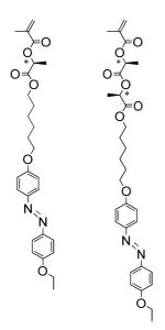
(S)-ML6A (S,S)-MLL6A Figure 10: Structures of the monomers (S)-ML6A and (S,S)-ML6A
