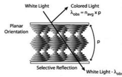
Figure 1: planar alignment and selective reflection
