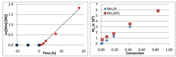
Figure 20: Kinetics of two step temperature polymerization with 30% of AIBN decomposition, red point on the plot are after decrease of temperature at  $40^{\circ}$ C
