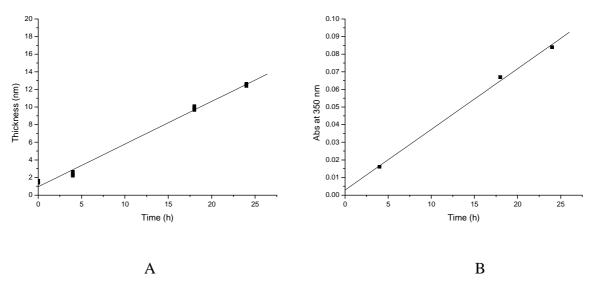
Figure 5. Kinetic plots of the SI ATRP of M6A in DMF (entry 5 in table 1) studied by ellipsometry on Si surfaces (A) and by UV-Vis spectroscopy on glass slide (B)
