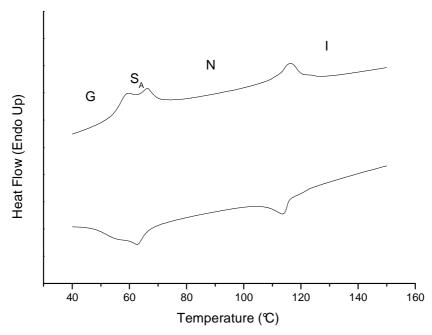
Figure 6: DSC cooling (first scan) and heating curves (second scan) for Poly(M6A)-8
