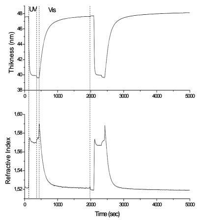
vertical lines indicate the UV and vis illumination switched alternatively on and off during the first cycle.
