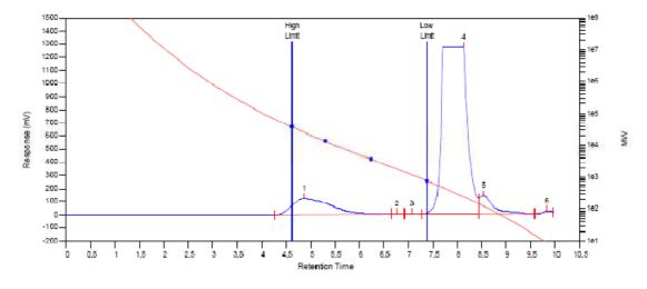
Figure 2: GPC chromatogharph of the polydisperse polymer in solution
