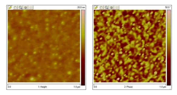
Figure 24 AFM images (topography and phase image) of PBA: PAA = 75: 25 after immersion in water and hexane.
