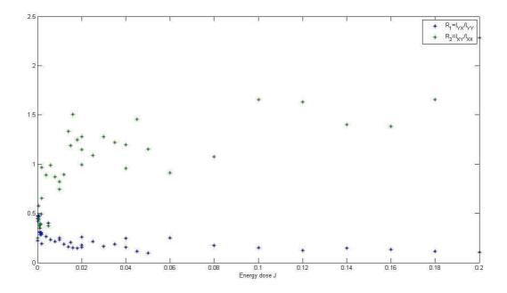
Figure 17: Scattering anisotropies  $R_1$  and  $R_2$  measured on the illuminated areas as a function of the energy dose in Joule of the pump beam.
