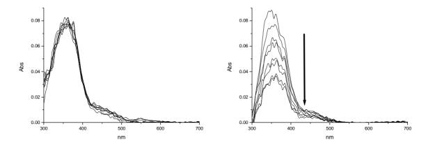
Figure 8: UV-Vis Isomerization kinetics of (a) Poly(M6A) brush and (b) spin coated film of Poly(M6A)
