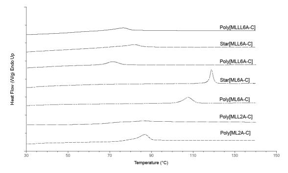
Figure 20: DSC traces of the second heating of the polymeric derivatives
