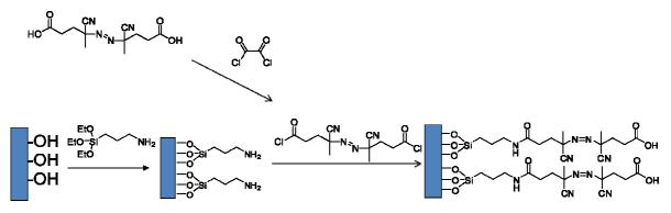
Scheme 2 functionalization of the surface with triethoxy silane and acylic chroride initiator
