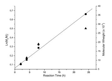
Figure 2. Evolution of  $Ln([M]_0/[M]_t)$  ( $\blacksquare$ ) and of the number average molecular weight determined by SEC in THF at 25°C ( $\blacktriangle$ ) and calculated values ( $\bullet$ ) versus time in the ATRP of (*S*)-ML6A in THF for Star[(*S*)-ML6A] series.
