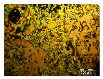
Figure 7. Polarizing optical micrographs of a typical schlieren texture of Poly(M6A)-8 in nematic phase after isotropisation and annealing at 100°C.
