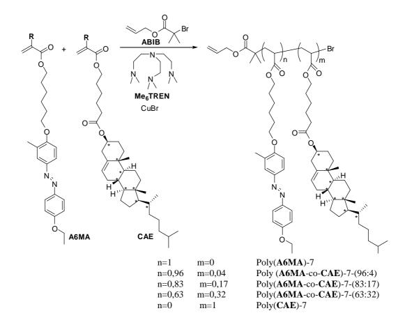
The polymerization procedure is as follow: the amount of reagent and solvent have been introduced under nitrogen flow in a vial and sealed. The oxygen have been removed with three freeze pump cycle and then CuBr have been introduced under vigorous nitrogen flow in the vial. Another freeze pump cycle had been then performed and the polymerization had been carried out at 80°C for 186 hours (7 days).
