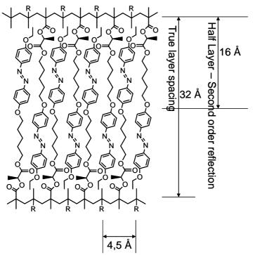
Figure 7. Smectic layer spacings of a fully interdigitated side-chain chromophoric configuration determined by XRD (R = chromophoric moieties located in the side chain outside the layer).
