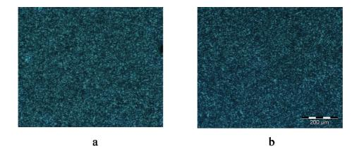
Figure 13 Optical microscopy images of a smectic thin film of Poly[(S)-**ML6A**]-14 before (a) and after irradiation with *l*-CPL for 30 minutes (b).
