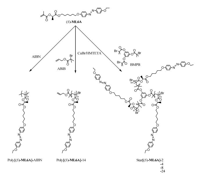
Scheme 2: Synthetic procedures and chemical structures of the (S)-ML6A polymers
