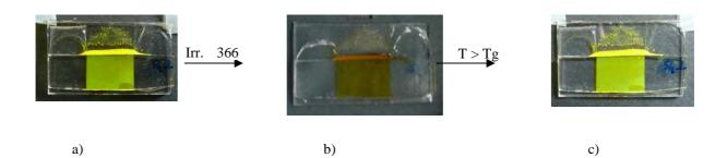
Figure 12. Smart label for the certification of thermal history
