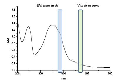
Figure 5: UV-Vis spectra of Poly(M6A)-8 and irradiation light
