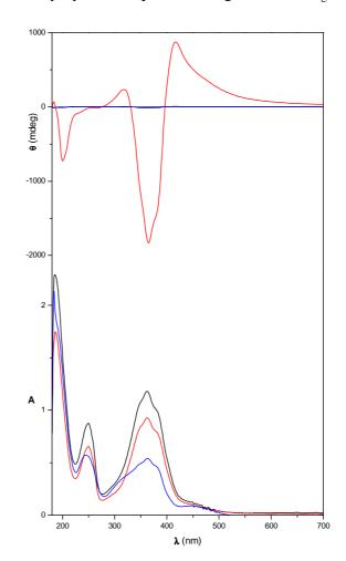
Figure 13. CD (up) and UV-Vis (down) spectra of a 200 nm thick film of Poly(M6A-co-CME)-1-(58:42) as casted film(—), after annealing at 100°C for 2 hours (—) and after irradiation at 366 nm for 4 hours (—)
