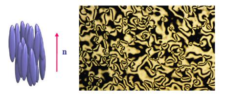
Figure 10: Schematic representation of the nematic mesophase(left) and typical texture corresponding, showed by Polarized Optical Microscopy(right)
