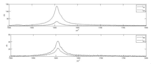
Figure 16: Raman peak of 5CB corresponding to the symmetric stretching of the benzene rings  $(1605 \text{ cm}^{-1})$  measured in the four geometries  $I_{VV}$ ,  $I_{VH}$ ,  $I_{HH}$ , and  $I_{HV}$ .
