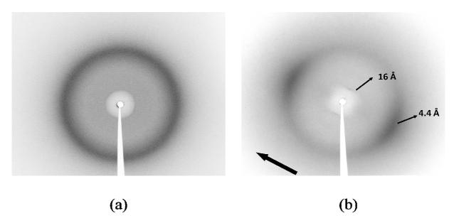
Figure 6: X-ray diffraction pattern of the SmA mesophase of Poly[(S)-ML6A]-14 recorded at room temperature after heating at 135°C (a) and oriented X-ray diffraction pattern of the SmA mesophase of Poly[(S)-ML6A]-14 recorded at room temperature (b). The sample was mechanically aligned in the direction of thick arrow.
