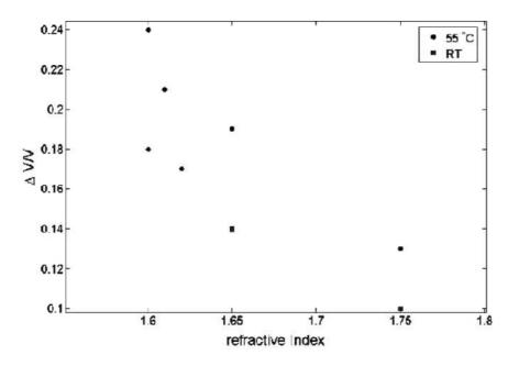
Figure 15: Correlation between expansion and refractive index (density), data acquired at 55°C (circles) and at room temperature (squares).
