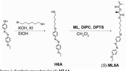
Scheme 1: Synthetic procedure for (S)-ML6A.
