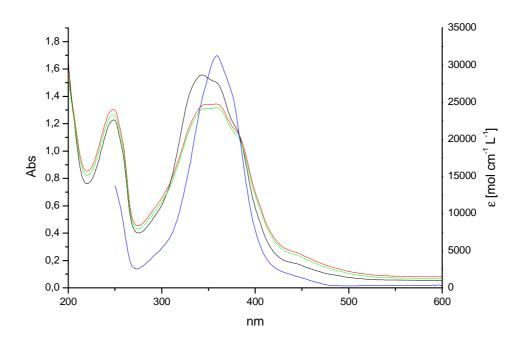
Figure 15: UV-Vis spectra of Poly[M6A]-24 in solution (—), and in the solid state as casted (—), annealed (—), and finally irradiated with l-CPL (—) thin films. The UV-Vis spectra of Star[M6A]-24 under the above conditions are superimposable.
