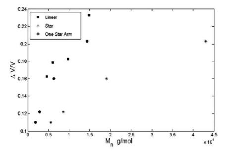
Figure 14: Percentage volume variation as a function of the molecular weight of the linear polymers (squares), Star Polymers (Stars) and of each branch ( $N_f=3$ ) of the Star polymers (Circles).
