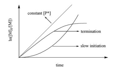
Figure 1 Illustration of the dependence of  $ln([M]_0/[M])$  on time
