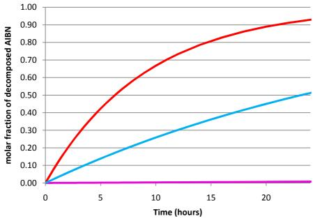
Figure 19: decomposition of AIBN at different temperatures (-) 70°C, (-) 65°C,(-) 40°C.
