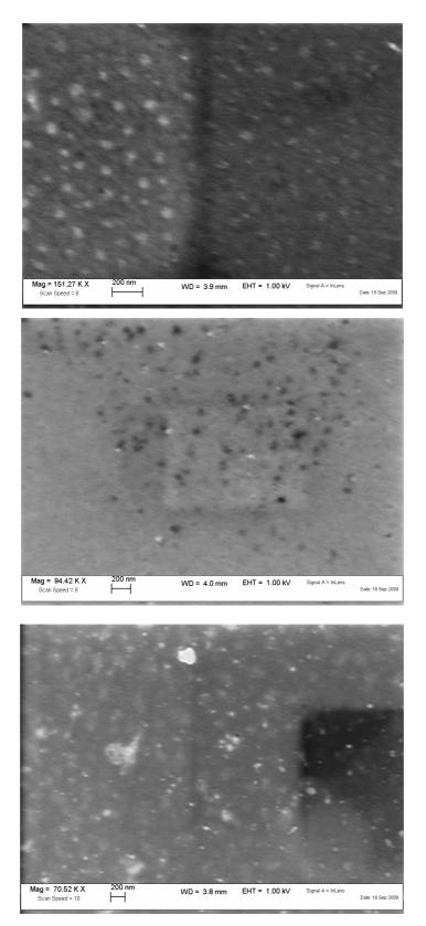
Figure 7: SEM images of M6A brushes on silica surface with different coverage of ATRP initiator after polymerization. SBiB: TMCS ratio (from top to down) = 1:1000; 1:50, 1:0
