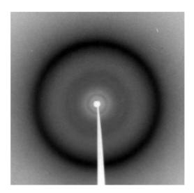
Figure 9: XRD diffraction pattern of Poly(M6A)-24 in the glassy smectic phase.
