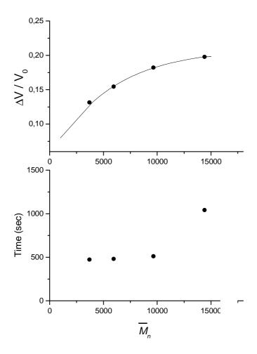
Figure 12: Photoinduced volume expansion (a) and relaxation times (b) versus the increment of sample average molecular weight after irradiation with 200  $\mu$ W/cm2 UV light (385 nm) at room temperature.
