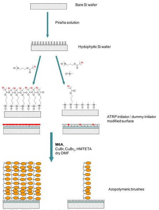
Figure 3: SI-ATRP of M6A from functionalized Si surfaces
