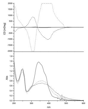
Figure 11: CD (up) and UV-Vis (bottom) spectra of a thin film of Poly[(*S*)-**ML6A**]-14 in the virgin state (—), in smectic phase (---) and after irradiation with *r*-CPL at 488 nm for 30 minutes (<sup>……</sup>).
