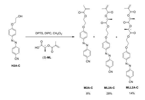
In a 150 ml three neck flask with magnetic stirrer, under nitrogen flow, 0,96 g of **H2A-C** (0,00362 mol), 0,57 g. of L-methacryloyl lactic ascid [(*S*)-**ML**] (0,00362 mol), 1,05 g of DPTS (0,00362 mol) e 0.2 g di 2,6-di-ter-buthyl-paracresole (polimerization inhibitor) and 11 ml of anhydrous  $CH_2Cl_2$  are introduced. To this solution under vigorous stirring 0,73 ml of N,N-di-isopropyl carbodimmide (DIPC) (0,00471 mol) are added.
