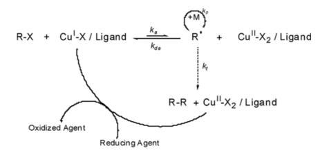
Scheme 5: ARGET ATRP mechanism
