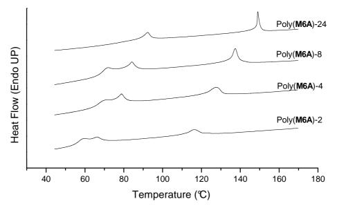
Figure 8: DSC heating curves (second scan) of the linear polymers investigated
