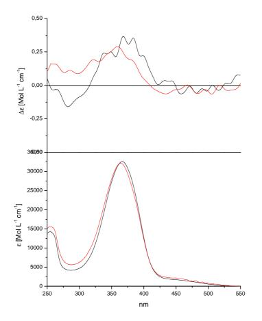
Figure 23. CD (up) and UV-Vis (bottom) spectra of (S)-ML6A-C (-) and of Poly[(S)-ML6A-C] (-) in chloroformic solution
