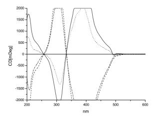
Figure 12: CD spectra of films of Poly[(S)-**ML6A**]-14 irradiated with *r*-CPL (-) or *l*-CPL (---) and Star[(S)-**ML6A**]-24 irradiated with *r*-CPL (-) or *l*-CPL (-.-) for 30 minutes after isotropization and annealing at 90°C for 15 minutes.
