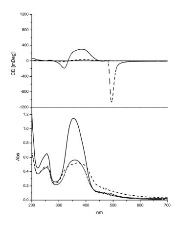
Figure 24 CD (up) and UV-Vis (bottom) spectra of thin film of Poly[(*S*)-ML6A-C] in the virgin state (—), after annealing (<sup>…</sup>) and after irradiation with *l*-CP (– –)
