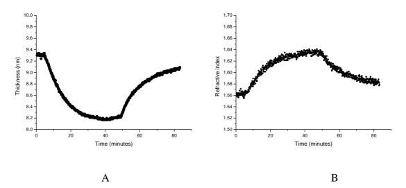
Figure 9: changing of thickness (A) and refractive index (B) of a Poly(M6A) brush under UV illumination (from 0 to50 mins) and Vis (after 50 mins).
