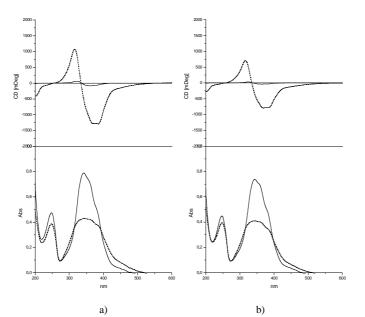
Figure 10. CD (up) and UV-Vis (bottom) spectra of a thin film of Poly[(*S*)-**ML6A**]-14 (a) and Star[(*S*)-**ML6A**]-24 (b) in the virgin state (-) and after isotropisation and annealing at 90°C for 15 minutes (- - -).
