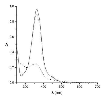
Figure 11. UV-Vis spectra of Poly(A6MA)-7 in CHCl<sub>3</sub>: (—) all *trans* isomers of the azoaromatic units, (---) after irradiation at 366 nm in order to reach a promote the *trans-cis* isomerization of azoaromatic chromophores, (····) after seven days in the dark at room temperature.
