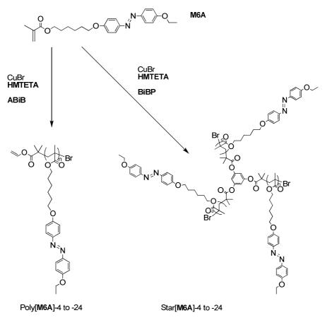
Scheme 1: Synthesis of linear and star-shaped polymeric derivatives
