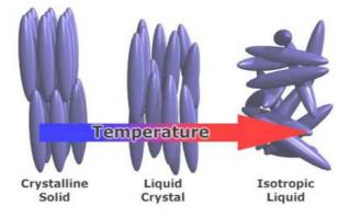
Figure 6 Average alignment of the molecules: a) solid phase, b) liquid crystal phase, c) liquid phase.
