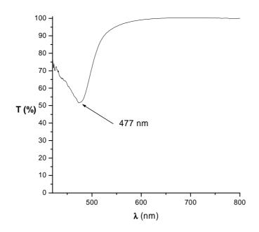
Figure 8. UV-Vis spectra of a 8,8  $\mu$ m thick film of Poly(M6MA-co-CME)-1-(58:42) in N\* phase without the contribution of the azoaromatic counits
