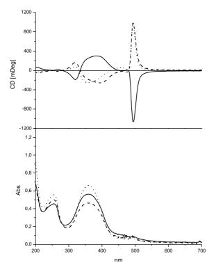
Figure 25. CD (up) and UV-Vis (bottom) spectra of thin film of Poly[(S)-ML6A-C] after irradiation with *l*-CP (\_\_\_\_), *r*-CP (- - -) and *r*-CP after a previous irradiation with *l*-CP (. . .)
