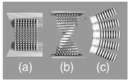
Figure 22: elastic deformation of a LC lattice a) splay, b) twist, c) bending)
