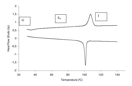
Figure 19: Thermogram of Poly[(S)-**ML6A-C**] under nitrogen atmosphere, at a heating and cooling rate of  $10^{\circ}$ C/min. G = glassy state, S<sub>A</sub> = Smectic A phase, I = isotropic phase.
