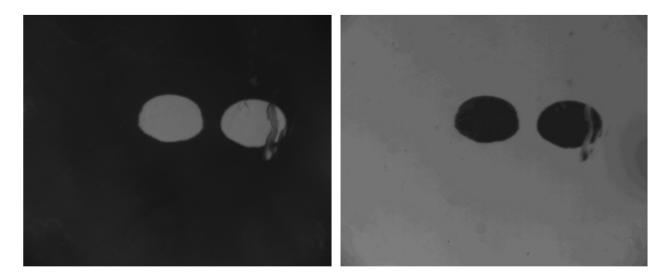
Figure 14: Polarizing microscopy images of 20  $\mu$ m diameter planar structures in a twisted cell. Left and right images have been acquired respectively with parallel and crossed polarisers.
