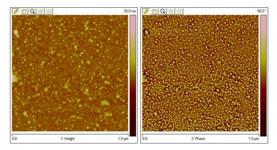
Figure 25 AFM images (topography and phase image) of PBA: PAA = 25: 75 after immersion in water and hexane.
