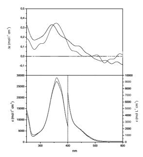
Figure 9. CD (up) and. UV-vis (bottom) spectra of (S)-ML6A (---) and Poly[(S)-ML6A]-14 (---) in CHCl<sub>3</sub>.
