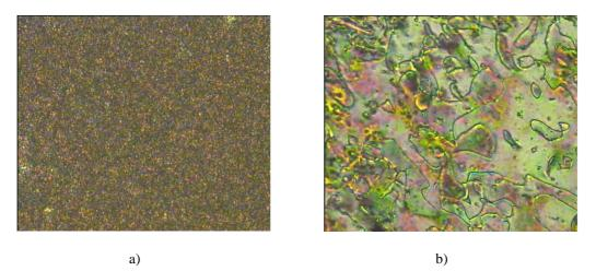
Figure 5. POM microphotograph, 32x magnification, of Poly(A6MA)-7 at 40  $^\circ C$  (a) and at 75  $^\circ C$  (b) after isotropization
