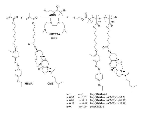
The procedure of the synthesis and purification of these derivatives is the same as the acrylic derivatives except that the polymerization were carried for 24 hours at 60°C and the polymers were precipitated in cold methanol.
