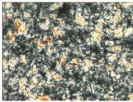
Figure 6: POM microphotograph, 32x magnification, of Poly(CME)-1 at 90°C after isotropization
