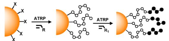
Figure 5: Modification of nanoparticles by SI-ATRP
