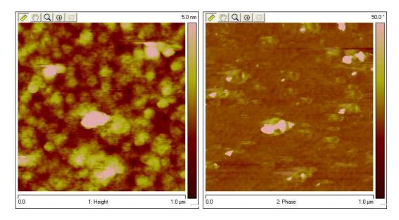
Figure 23: AFM images (topography and phase image) of PBA: PAA = 50: 50 after immersion in water and hexane.
