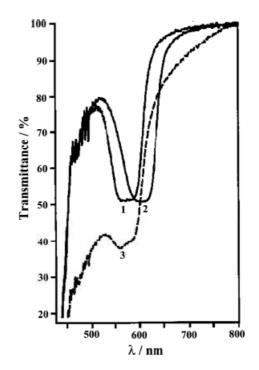
Figure 4. Shift of the Bragg reflection in the thermodynamically stable state (1), after 10 minutes of irradiation with UV light(2) and after 30 minutes (3).
