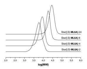
Figure 3. Normalized molecular weight distributions of Star[(*S*)-**ML6A**] polymers as determined by SEC in THF at 25°C.
