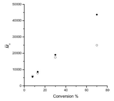
Figure 4: Evolution of the number average molecular weight determined by SEC in THF at  $25^{\circ}$ C (o) and calculated values (•) versus conversion in the ATRP of M6A.
