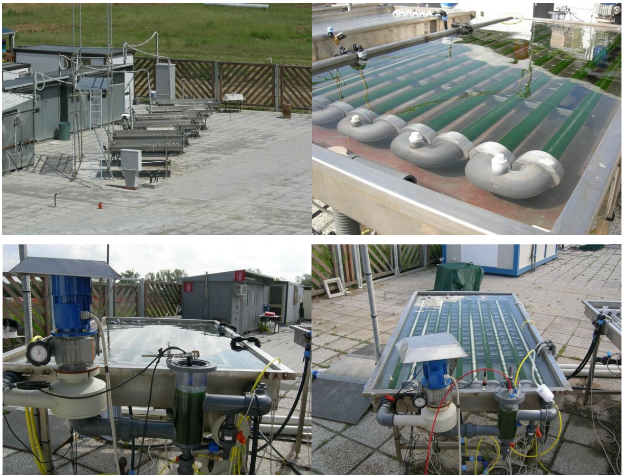
Figure 13. General overview of the outdoor PBR (clockwise): Panoramic view of the outside area, with six parallel 50-liter horizontal tubular outdoor PBRs; Particular of the tubular outdoor PBR during hydrogen production experiments; Picture showing the overall PBR system; Particular of the PVC pump for culture mixing and of the degasser.
