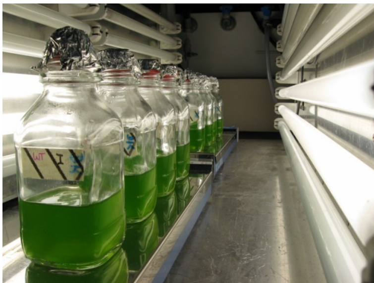
Figure 26: Overview of the final set up for the \text{H}_2 production in sulfur deprivation with sealed PBRs. Light intensity was provided by both sides and adjusted at about 60-70 \mu\text{mol photons m}^{-2} \text{s}^{-1} . Initial chl concentration was 12 \text{mg L}^{-1} and PBR volume was 325 mL. The working volume of the reactor was 115 mL, with the remaining part (210 mL) being gas phase. PBRs were operated at room temperature (20-25 ^\circ\text{C} ). Cultures adopted in this set of experiments were cultivated in photoheterotrophic conditions at 20 ^\circ\text{C} .
