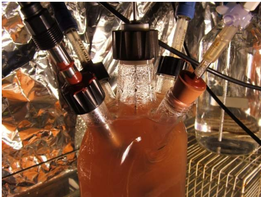
Figure 15. H 2 production experiments by means of photo-fermentative processes carried out with purple non sulfur bacteria, using the impeller mixing device developed by us.
