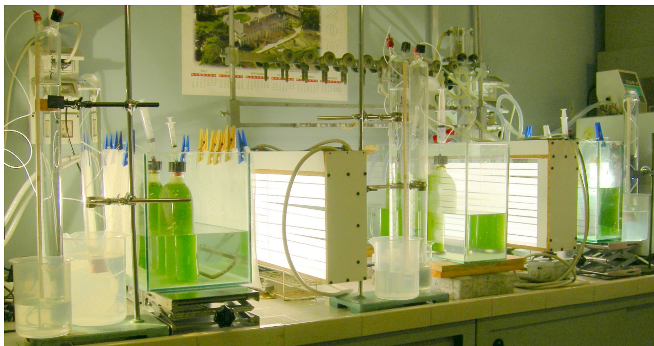
Figure 1. A panoramic view of the screening system adopted for the H 2 production under sulfur deprivation. Initial chl content was set at 12 mg L -1 , initial pH was 7.2. Cultures were irradiated with 70 μmol photons m -2 s -1 per side. Temperature was adjusted at 28°C by placing PBRs in a bath filled with deionized thermo-stated water. Mixing was allowed by a magnetic stir bar placed at the bottom of the PBR. Biogas production was evaluated by water displacement.
