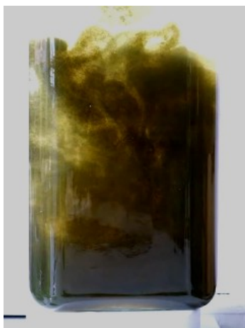
Figure 8. Boundary level relative to a fully turbulent mixing in a stir bar-mixed PBR with a flat cross section. Fluid was colored by means of black dye addition at the bottom of the PBR, near to the rotating stir bar. Note that black dye stops at about 3/4 of the PBR height. Blobs of traced liquid propagating irregularly like a cloud, responsible for the spikes noted in Fig. 7 with NaCl solution, can also be appreciated.
