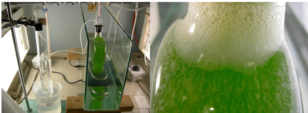
Figure 5. Hydrogen production experiment with the screening system set up (left) and particular of the Roux-bottle type PBR during H 2 gas evolution (right). After saturating the liquid suspension, the H 2 gas is collected as foam and bubbles in the upper part of the PBR.
