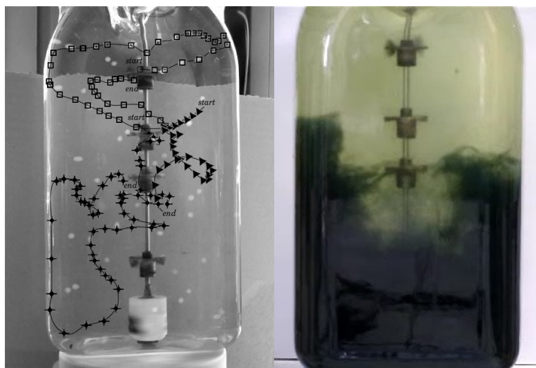
Figure 6. (Left) Photograph showing some real fluid trajectories of selected tracer particles produced by the multiple-impeller stirring device, and (right) spatial distribution of black dye drops added at the bottom of the impeller-mixed PBR. Note on the right picture the loop created at the third turbine (from the top), which clearly demonstrates the liquid exchange between the outer and the inner zone of the PBR.
