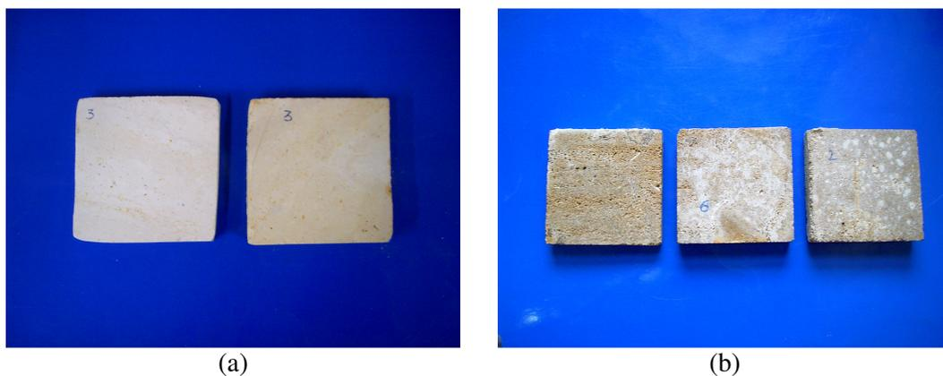
Fig. 143. Laspra treated with Tegosivin HL 100 before and after the exposure to  $SO_2$  action (a); Repedea treated with Silres® BS 290 and TMSPMA before and after the exposure to  $SO_2$  action (b)
