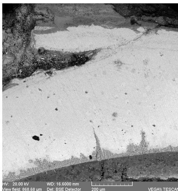
*Figure IV.36: BSE-SEM micrograph of the stratigraphical section of the arrowhead. Overview of corrosion layers: as it is commented in the text, the surfaces differ in the internal and in the external side of the section.*
