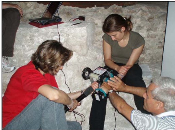
Fig. 5-3: Application of DRMS in-situ
