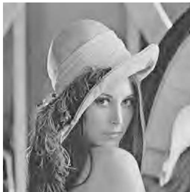
(b) Received Image. R_{rcpc} = 0.33, R_{rs} = 0.99, \text{PSNR} = 29.0 \text{ dB}, R_{\text{TX}} = 0.08 \text{ bpp}, R_{\text{RX}} = 0.073 \text{ bpp}.
