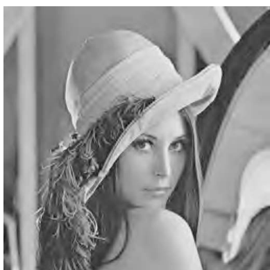
(c) Received Image. Optimal Rate. R_{rcpc} = 0.5, R_{rs} = 0.89, \text{PSNR} = 30.5 \text{ dB}, R_{\text{TX}} = 0.15 \text{ bpp}, R_{\text{RX}} = 0.1 \text{ bpp}.
