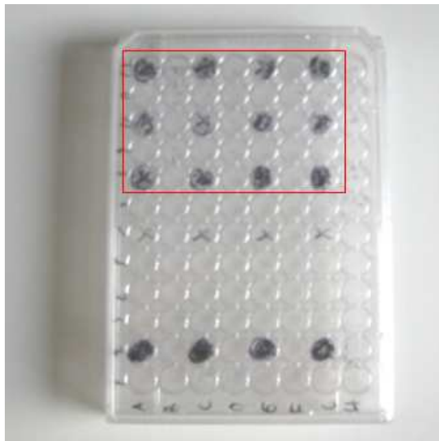
Figure 1.1: A picture of the wells used to assess biological response to ^{188}\text{Re} of a set of human tumor cell lines. The rectangle indicates the well geometry used in the MC simulation (see Section 1.4).
