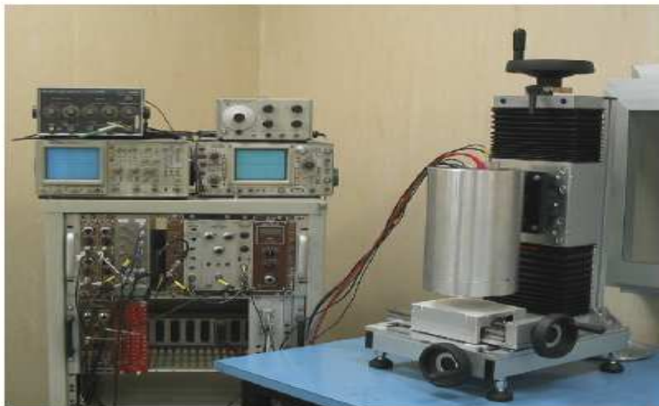
Figure 1.17: The experimental apparatus which is taking data at INFN in Legnaro (Padua - Italy). On the right one can see the mechanical structure and source positioning system, which contains the scintillator, the PM and the collimator inside the cylinder. The rack containing the readout electronics is visible on the left.
