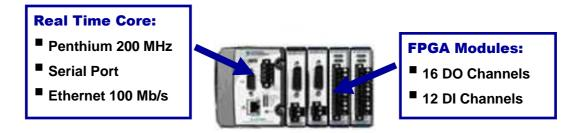
Figure 3: National Instruments CRIO Onboard Computer
