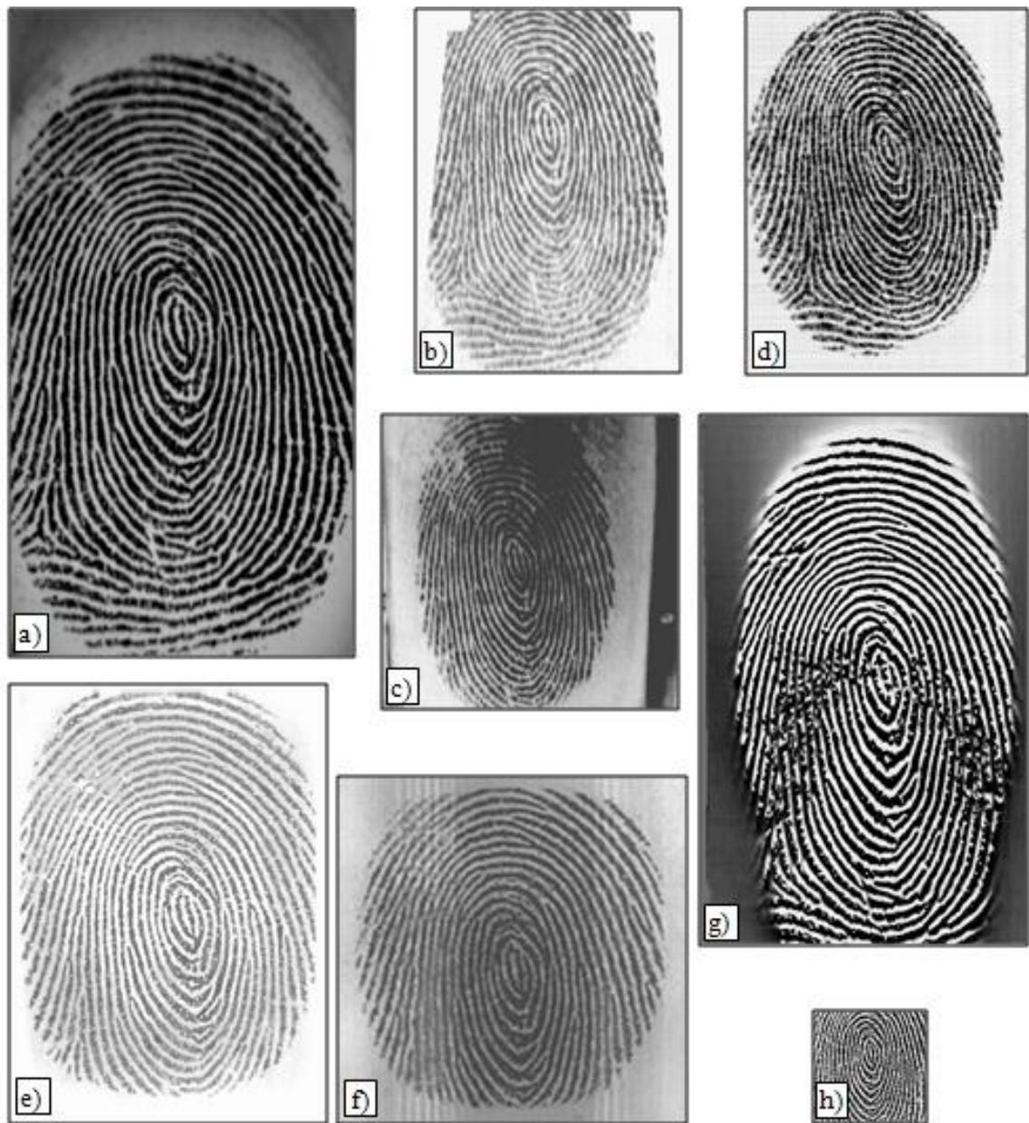
Figure 2.3 – Fingerprint images of the same finger as acquired by different commercial scanners. Images are reported with right proportions: a) Biometrika FX2000, b) Digital Persona UareU2000, c) Identix DFR200, d) Ethentica TactilSense T-FPM, e) ST-Microelectronics TouchChip TCS1AD, f) Veridicom FPS110, g) Atmel FingerChip AT77C101B, h) Authentec AES4000 [9].
