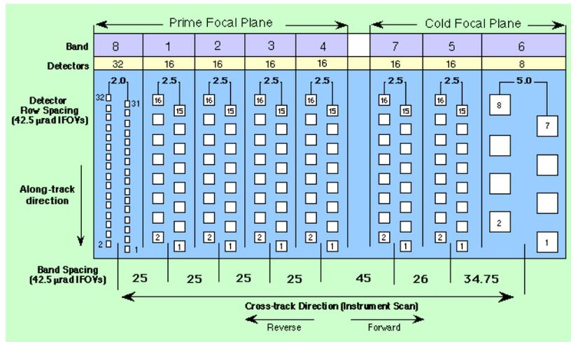
FIGURE\_4.9: Detector Projection at the Prime Focal Plane
