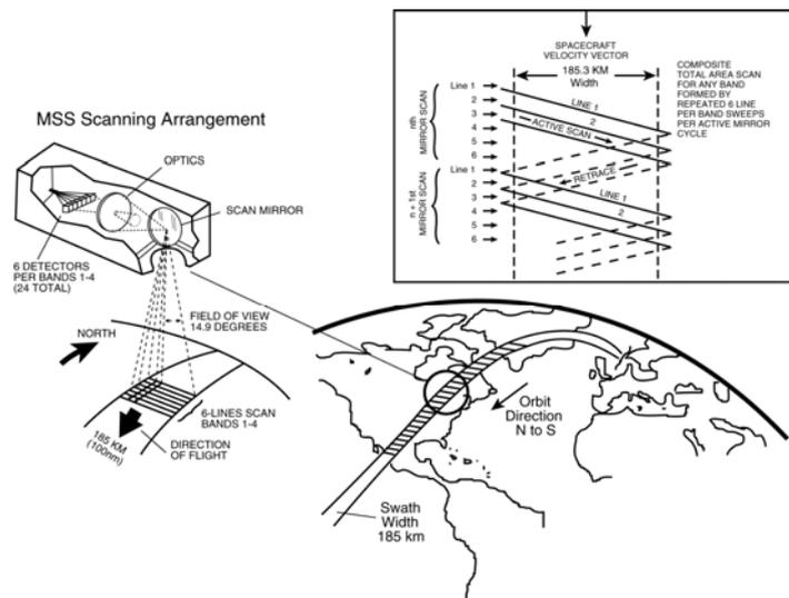
FIGURE\_4.4: MSS Scanning system [130]
