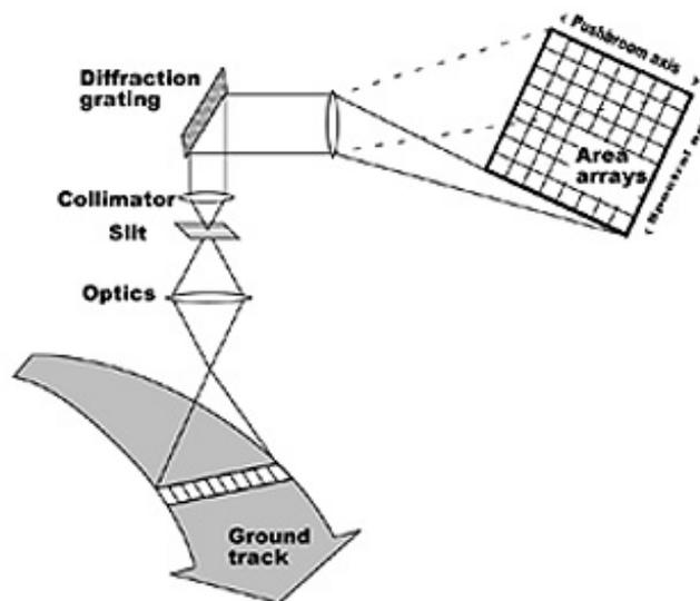
**FIGURE\_4.11: Scheme of a pushbroom scanning**
