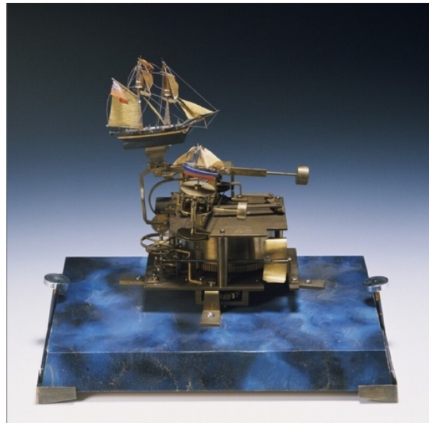
Fig. 1.11. Mechanism reproducing the movement of boats in the sea by Crevier and Piolaine (around 1880). © Musée des arts et métiers.
