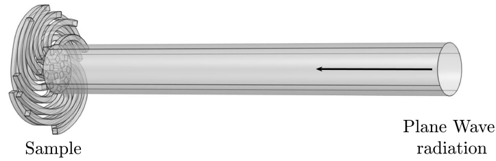
Fig. 4.4 Schematic drawing of the numerical model to simulate the acoustical behavior of the multi-resonant metamaterials. The openings of the QWRs are positioned across the available area of diameter 2 cm, while the cavities are developed on two levels, utilizing the entire available space within the tweeter's enclosure.
