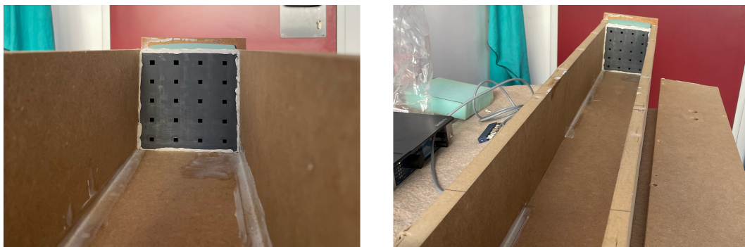
Fig. 3.11 Pictures of the sample mounted inside the square-based impedance tube.
