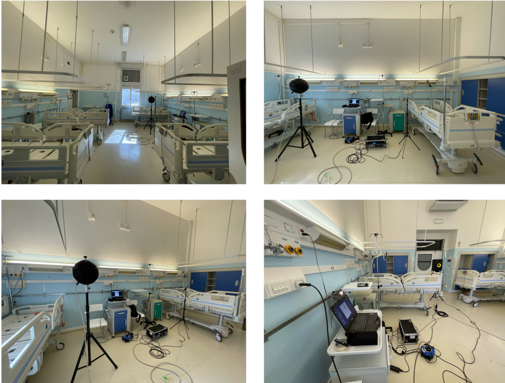
Fig. 3.5 Photographs of the reverberation time measurements in the empty room: an omnidirectional source (dodecahedron) has been used as a source in two locations.
