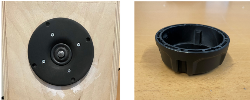
Fig. 4.1 Photographs of the tweeter under study: on the left, a frontal view of the tweeter featuring the flange, the waveguide, and the diaphragm. On the right is the enclosure that separates the rear of the tweeter from the surroundings.
