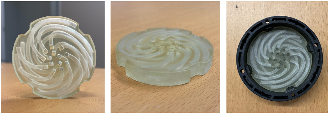
Fig. 4.7 Pictures of the metamaterial sample produced in resin through Stereolithography (SLA). The sample has a thickness of 8 mm and has been designed to be placed inside the tweeter's enclosure.
