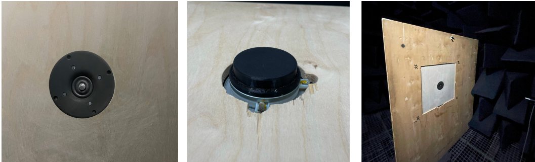
Fig. 4.8 Photographs of the tweeter mounted in the baffle for frequency response measurements: (Left) the front view of the tweeter; (Center) the rear view of the tweeter; (Right) Measurement setup used in the anechoic chamber, including the tweeter in the baffle and the microphone at a distance of 25 cm.
