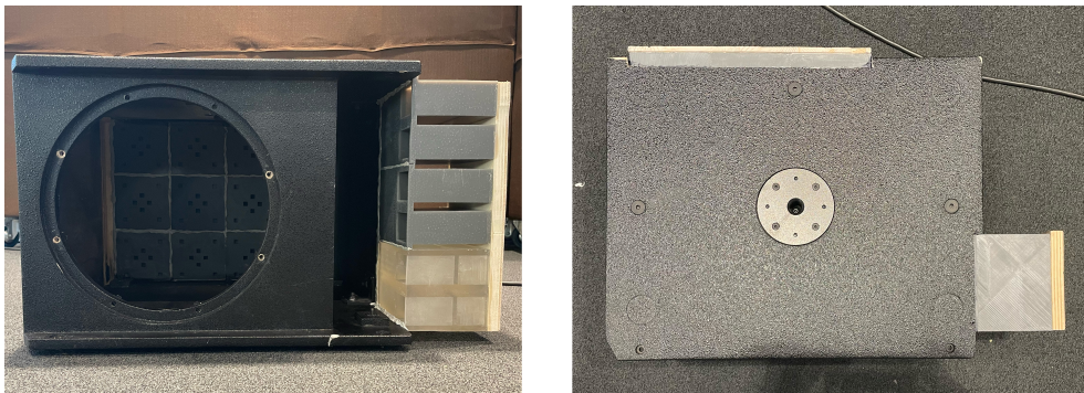
Fig. 4.26 Photographs of the metamaterial panel for the zero transmission. The panel is the array 3x1 of the single unit cell for absorption located in the bottom panel of the reflex.
