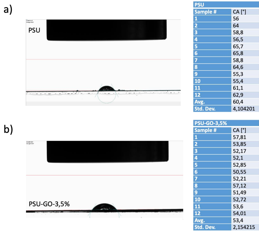
Fig. 8.19. Contact angles values and images of PSU and PSU-GO 3.5% HF. Contact angle of PSU-HF and PSU-GO 3.5% HF were measured with OCA Dataphysics instrument. Fibers were flattened before measurement to remove the outer porosity of the fiber and allow the measurement of the contact angle of the material.
