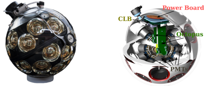
Figure 34: Left: picture of the KM 3 NeT digital optical module. Right: schematic representation of the components inside a DOM. Taken from [84].
