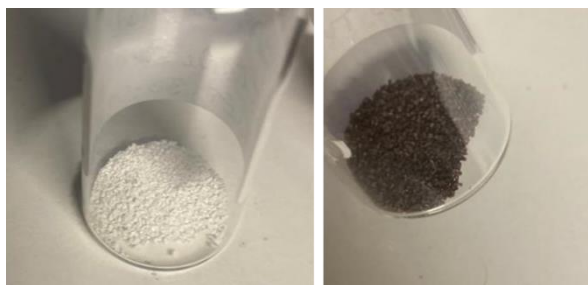
Figure 26. Tetragonal zirconia catalyst pre (left) and post (right) reaction of CTH of ML to GVL
