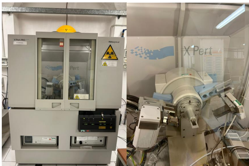
Figure 17. Philips X'Pert vertical diffractometer instrument for XRD analysis
