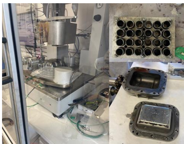
Figure 56. SPR pressure reactor from RealCat Lab and 24 reactor plate
