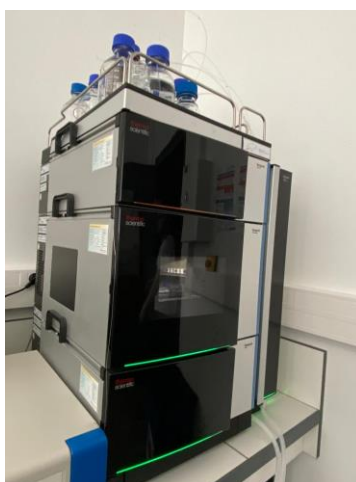
Figure 86. Shimadzu HPLC used of the quantitative analysis of HMF oxidation
