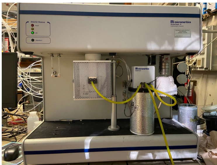
Figure 19. Autochem II- Micrometrics. Chemisorption analyzer
