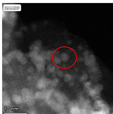
Figure 71. TEM image of Pd 0.5%wt/ ZrO_2 (61192). In the red circle a Pd nanoparticle is highlighted.
