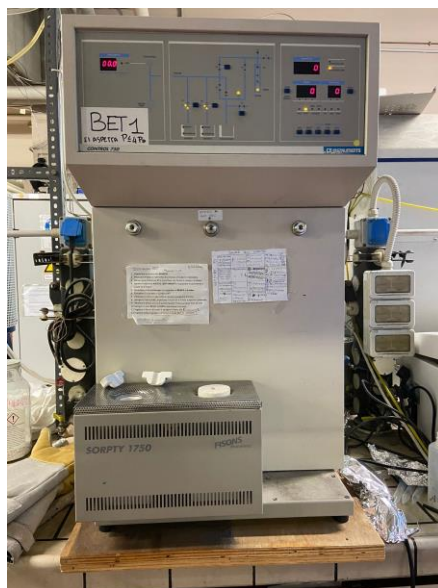
Figure 18. Instrument Sorbity 1750 for BET surface analysis
