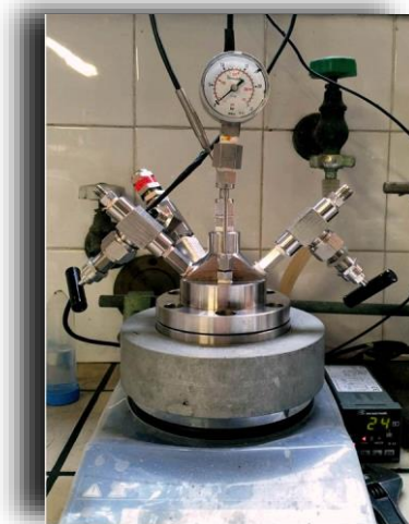
Figure 101. Autoclave reactor used for glucose oxidation.
