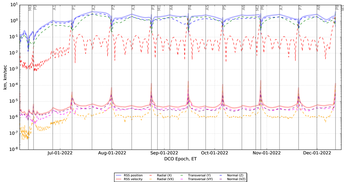
Figure 4.32: Evolution of the expected S/C ephemeris uncertainty ( 3\text{-}\sigma , Earth-centered RTN frame) through the whole mission after a REV by REV single-arc reconstruction.
